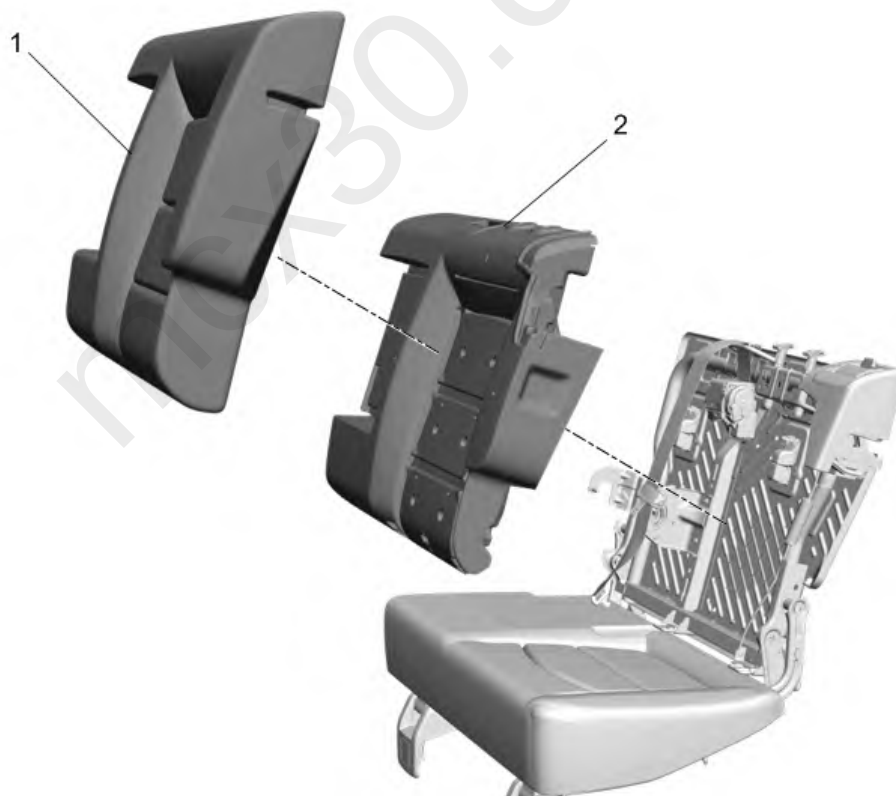
Fig. 77: Rear Seat Back Cushion Cover And Pad
